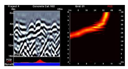
Power cables embedded in concrete pose an immediate risk when construction work needs to be done.
